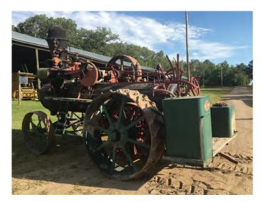
This 17-hp George White steam traction engine, manufactured in Canada as a portable power unit for belt work, would move from farm to farm with a separator in tow. It is fully operational, the first to enter museum collections since 1993.
